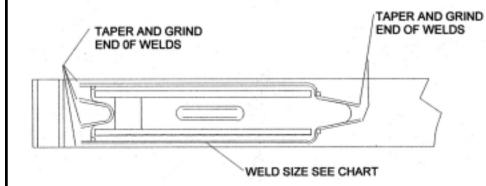
or equivalent electrode. All welding to be performed by a qualified or certified welder. See the bracket welding for detailed instructions. Welding to be peened and the end of each weld ground and tapered to eliminate weld stress and stress risers.
